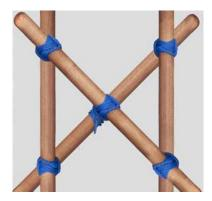
**Use**: The Diagonal Lashing is used to lash two spars together. Unlike the Square lashing which works for right angle crossings, the diagonal lashing secures poles crossing each other at a variety of angles. When the angle between the poles is closer to 45 degrees, the diagonal lashing is more appropriate.
