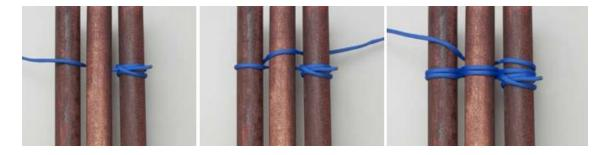
**Frapping Turns:** The turns surrounding the lashing at right angles exert a tightening effect on the lashing. These turns are known as Frapping Turns.
